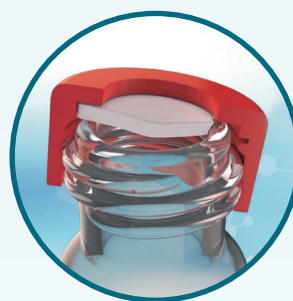
Cap tilt and septum displacement due to over tightening
